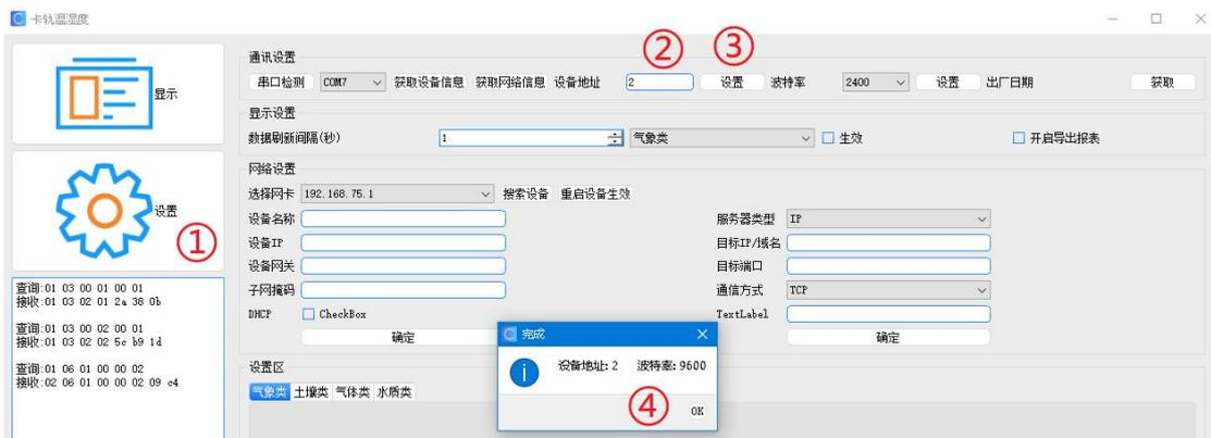
Modify the baud rate Steps: ①Set --- ②Select baud rate --- ③Set --- ④OK
